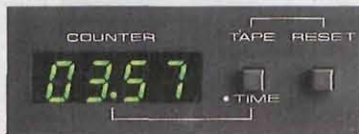
The real-time counter reads out the amount of tape left in meaningful minutes and seconds instead of meaningless inches.
